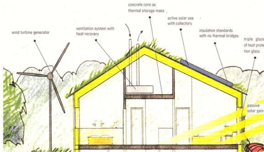
Principle of a 'Lummerland' passive house
